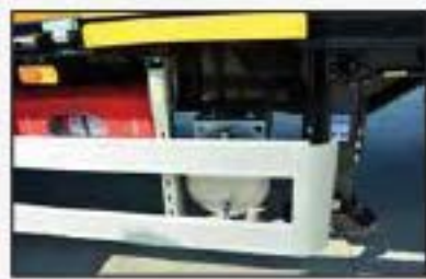
Side underrun guard, Landing gear, Water tank and Fire extinguisher
